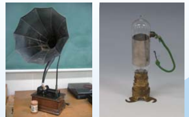
Edison phonograph, An early version of Fleming valve from UEC Museum of Communications
